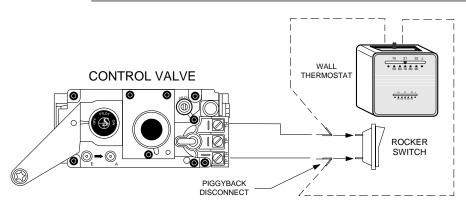
Remember the Rocker Switch must be turned to "OFF" while using the Wall Thermostat.
